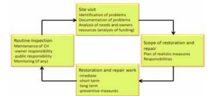
Figure 3.3.3.1: Planning for restoration and repair measures after flooding.
