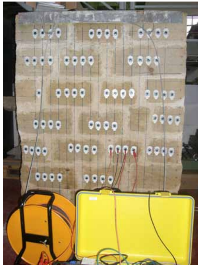
Figure 7.4.2.1: Field size CR measurements on a sandstone testing wall (left). Ordinary medical ECG electrodes are used. This picture shows a four-point Wenner setup. The water distribution was investigated after the wall was flooded for about a week. The results of Wenner ( a = 5 cm) measurements of electrical resistivity obtained on single stones are shown on the right. Source: BAM.
