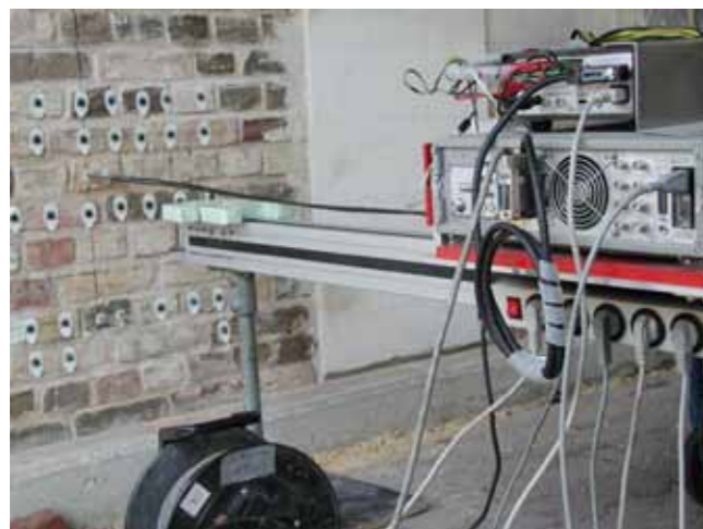
Figure 7.4.2.2: Left: Schematic presentation of the microwave borehole system (. Right: photograph of the microwave borehole transmission technique applied to a masonry specimen. Source: BAM.
