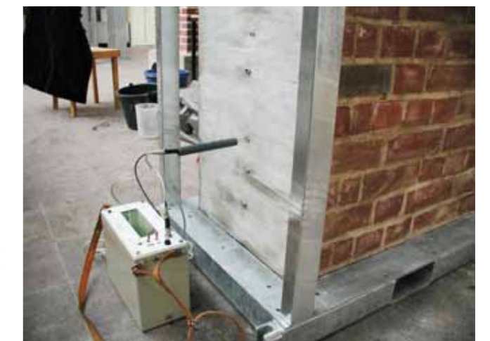
Figure 7.4.2.4: Left: Schematic diagram of a 2-rod probe consisting of two parallel metal rods of defined length. At discontinuities such as the beginning and the end of the metal bars the electromagnetic pulse is reflected. ( t_0 , t_1 und t_2 ). The signals are depicted for both a step pulse (grey) and a sine-shaped peak pulse (black). Source: Plagge (2003). Right: Photograph of the TDR technique being applied to a masonry specimen. Source: BAM.
