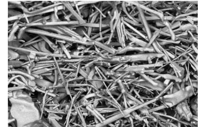
Figure 4.7.2.6: Lengthy needle-like halite crystals are the most frequent cause of degradation of the materials inside the church. Source: ZAG.
