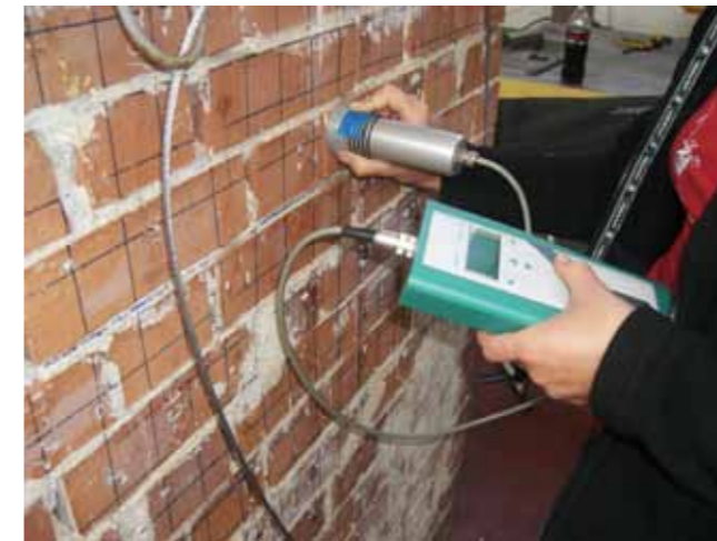
Figure 7.4.2.3: Left: Photograph of the microwave surface sensor being applied to a masonry specimen. Right: Results in terms of the moisture index obtained on a wet basement wall. The source of the water is located in the lower right corner. Source: BAM.
